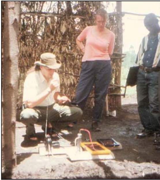
A DIY Solar module charging a torch/powerpack and simultaneously powering a radio.
